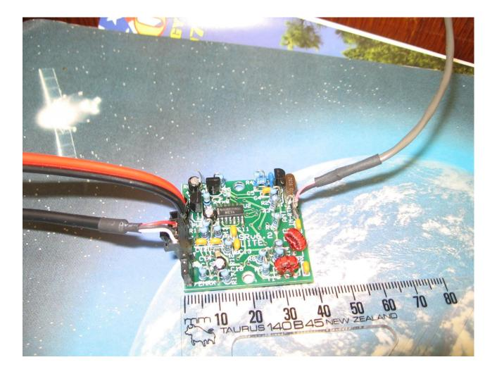
On reading about the SoftRock kits I reasoned that if I could set the device to work at the centre of the 9MHz 1<sup>st</sup> IF in my FT-301 receiver, I would be able tune to any frequency and still get the advantages of the SDR software. This would effectively add IF DSP filtering, band scope and demodulation to the old receiver. These are features usually only found in the latest top of the range transceivers.
